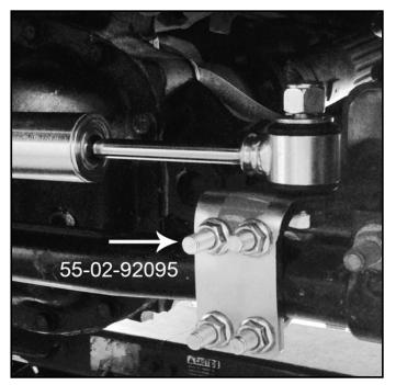
□ Attach the body end of the stabilizers to the top of the center axle bracket with the supplied 1/2" x 2-1/2" bolts, washers and nyloc nuts. The bolts should be inserted from the bottom. Snug but do not tighten the cylinders. Once the cylinders are in place, level the center axle bracket and tighten (30).
